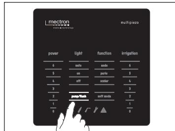
While the PUMP/FLUSH writing flashes, press the foot pedal once and release it, the PUMP/FLUSH stops flashing and the irrigation circuit begins to be filled up;
