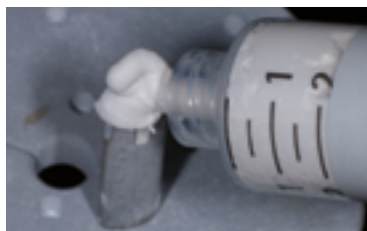
Appliquer IPS Object Fix Flow sur la tige IPS e.max CAD Crystallization Pin.
