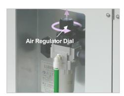
1. Pull up the dial on the air regulator and turn it until the pressure drops to 0 MPa.
