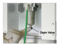
2. Put a container under the regulator and then press the drain valve.
