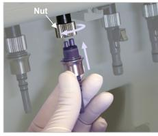
2. Fit the replacement coupling onto the nozzle and tighten up its nut.
