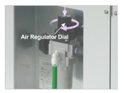
3. After draining the regulator, turn the dial back to adjust the pressure and push it back down.
