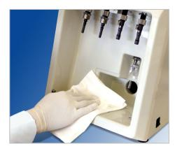
4. Clean the main body with a neutral detergent or ethanol for disinfection (Ethanol 70 to 80 vol%).
